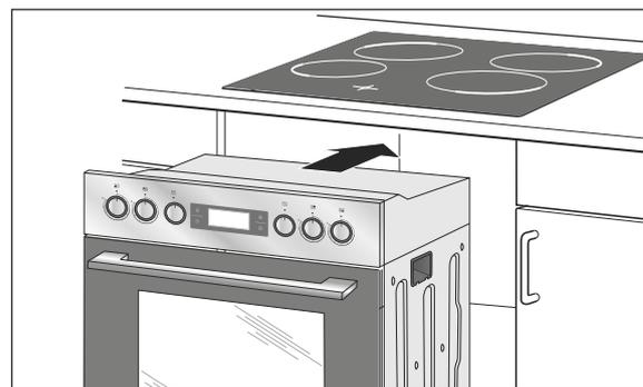
2. Use the carrying handles on the side of the oven to lift it and then push it as far back into the built-in cabinet so that the
