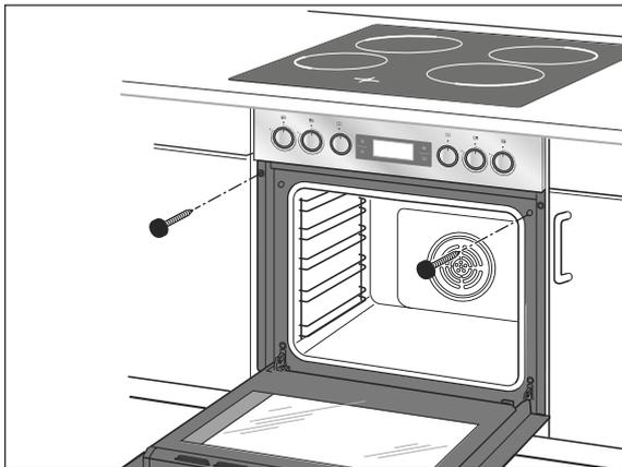
6. Screw the oven to the built-in cabinet with the two screws which have been supplied.
