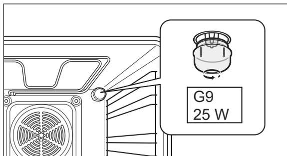
3. Unscrew the glass cover anticlockwise and remove it.
