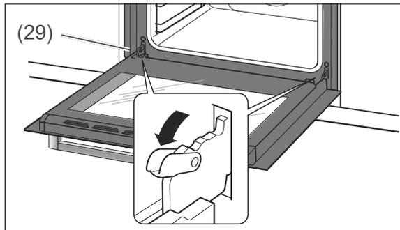
2. Fold the clips (29) on both sides all the way forward. Use a screwdriver if necessary.
