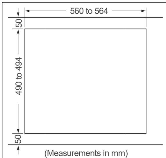
2. If a hob was already installed, the cut-out section must be no larger than:
