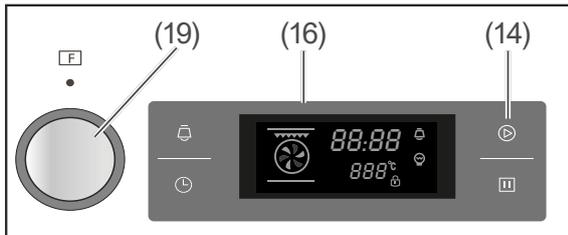
1. Selecting a function: Turn the dial (19) until the display (16) shows the corresponding symbol and its standard temperature.
