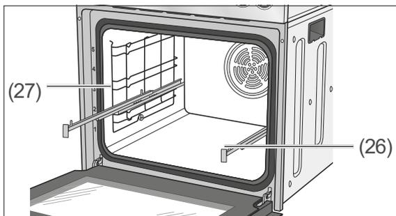
The side walls of the cooking compartment are equipped with oven rack guides (27) with telescopic oven rails (26). These make it easier to remove baking trays from the oven, for example, to baste roasts.
