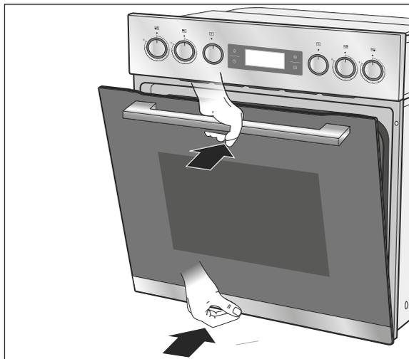
4. With both hands, lightly lift and guide the door forward out of its hinges.
