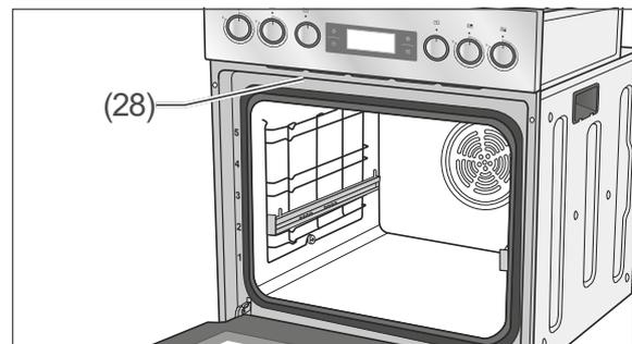
The external cooling fan cools down the steam and vapour that exit the oven through the extraction hood (28) and prevents adjacent units from becoming too hot.
