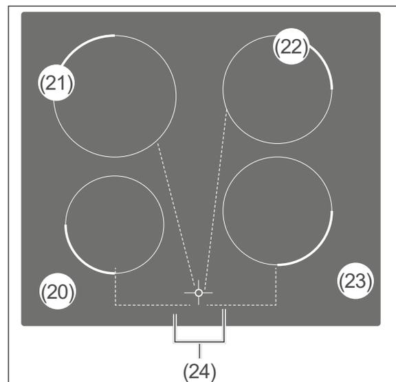
The residual heat indicators (24) indicate that surfaces are hot to prevent you from burning yourself. The H symbol indicates which of the cooking zones are hot.
