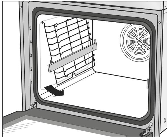
2. Pull the bottom of the oven rack guide approx. 45° away from the wall so that you can remove it.
