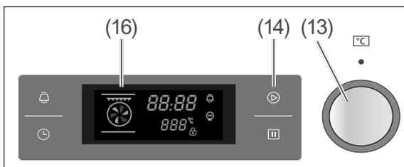
5. Adjusting the temperature: Turn the dial (13) until the display (16) shows the desired temperature.
