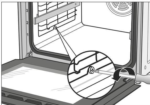
1. Loosen the screws on the oven rack guides and remove them.
