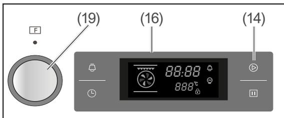
3. Changing the cooking time: Turn the dial (19) until the display (16) shows the desired cooking time (0:00 to 9:00).
