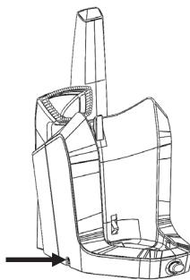
1. Separate the back part of the charging station from the front part by pushing it downward. (Fig. 1)
