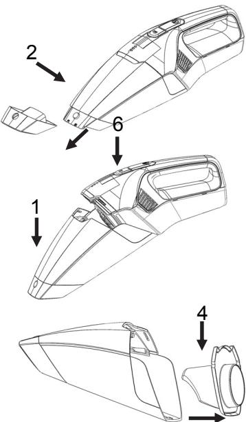
1. To empty the dust container, press the release button (2) and remove the suction nozzle. Then you can easily empty the container into the household trash. If the vacuum power decreases, you should clean the dust filter (4).
