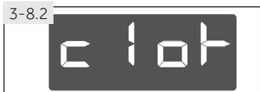
The display shows **c lot** (Fig. 3-8.2) if a button will be pressed, when the child lock is activated. The change is not running.
