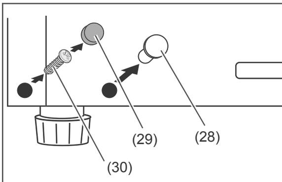
19. Lever out the blind plugs (28) and the cover cap (29) and loosen the screw (30).
