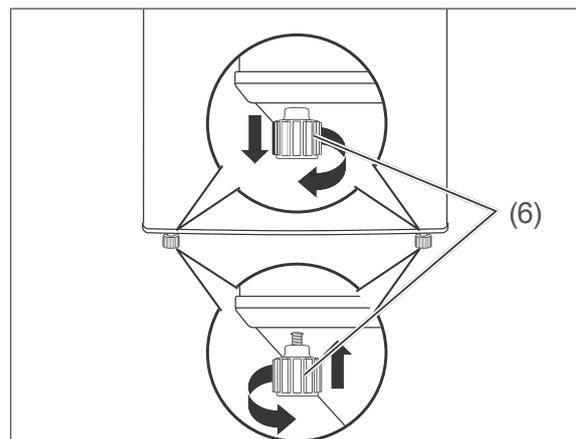
3. Level out any unevenness on the ground using the two front screw feet (6).
