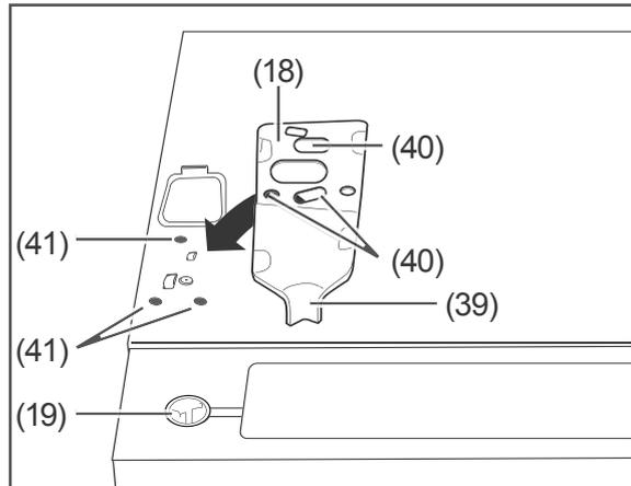
5. Insert the upper hinge (18) so that the hinge pin (39) slides into the plastic insert (19) and the screw holes (40) lay over the holes (41) in the appliance casing.
