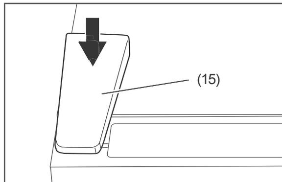
6. Reinsert the blanking plate (15) on the hinge side.
