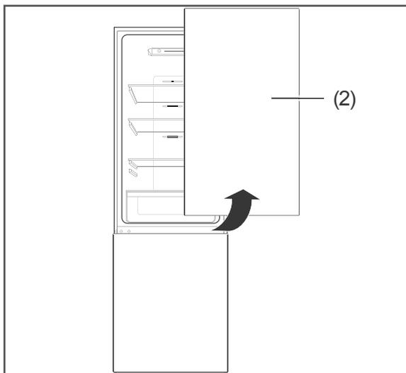
8. Lift the fridge door (2) out of the middle hinge fitting, and remove it.
