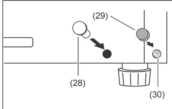
20. Fasten the screw, the cover panel and the blind plug on the opposite side.
