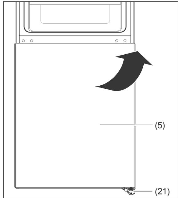
11. Lift the freezer door (5) out of the lower hinge (21), and remove it.
