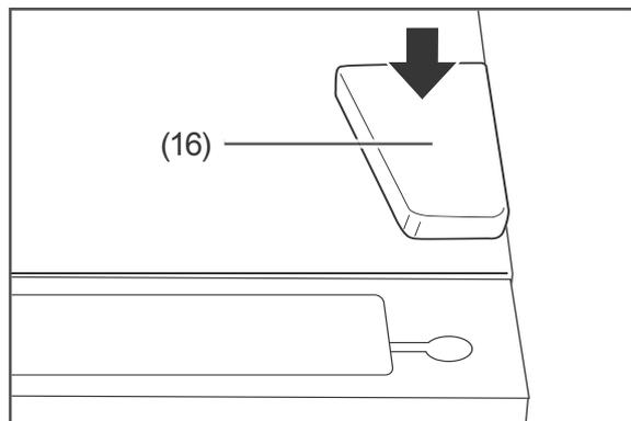
7. Reinsert the blanking plate (16) opposite the hinge side.
