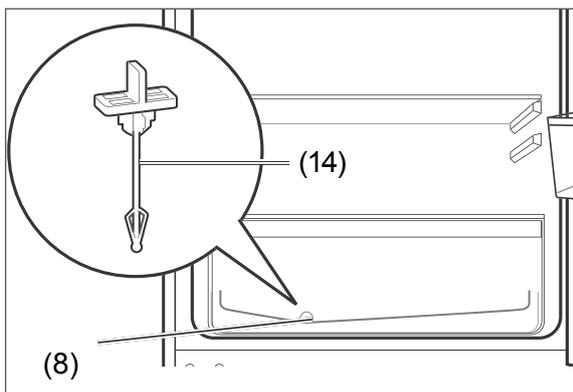
7. The defrost water drain (8) can be found on the reverse side of the refrigerator area behind the vegetable drawer. Clean the defrost water drain (8) with a cleaning tool (14).
