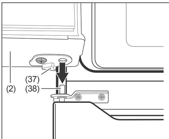
4. Reattach the refrigerator door (2) so that the top of the pin (38) slides into the hole in the metal reinforcement (37).
