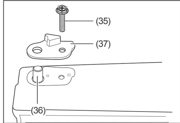
4. Insert the plastic sleeve (36) on the opposite side and use the screw (35) to screw the supplied metal reinforcement (37) on the opposite side.
