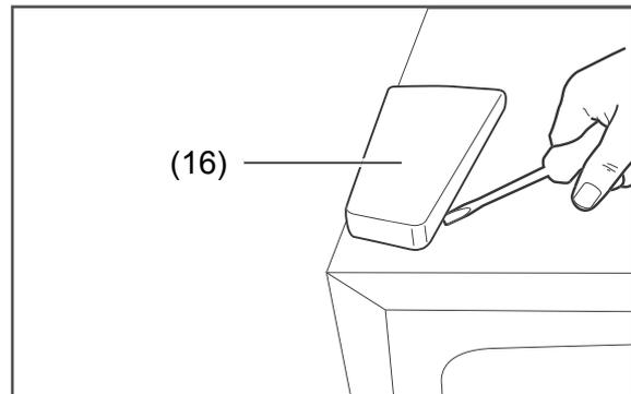
4. Lever the opposite blanking plate (16) upwards also and lift it off.
