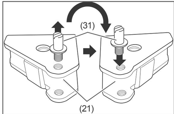
21. Unscrew the pin screw (31), turn the lower hinge over (21) and tighten the pin screw on the other side.
