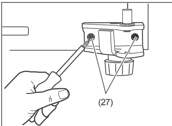
18. Unscrew both screws (27), and remove the lower hinge (21).
