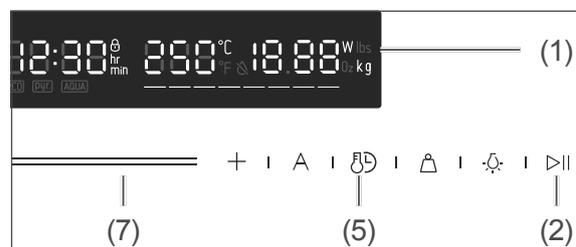
3. To change the temperature, use the +/- sensors or the slider (7).
