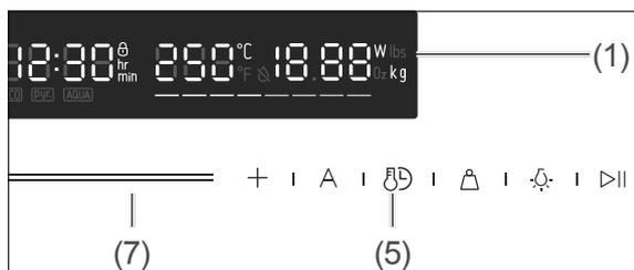
3. To change the cooking time, tap the
