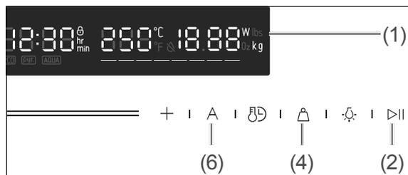
2. To select the automatic mode, tap the **A** sensor (6) until the display (1) shows the desired programme.
