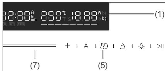
3. To change the cooking time, tap the sensor (5) and use the +/- sensors or the slider (7).
