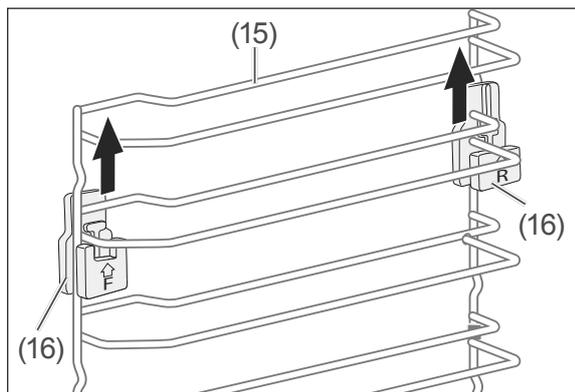
2. Push the baking tray guides (15) upwards out of the brackets (16).
