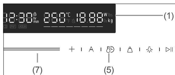
4. To change the temperature, use the +/- sensors or the slider (7).
