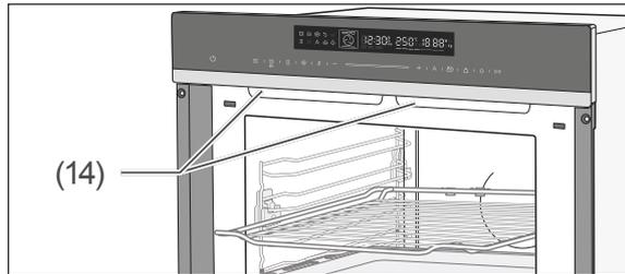
The air outlet is through the extraction hood (14) between the control panel and the oven door.
