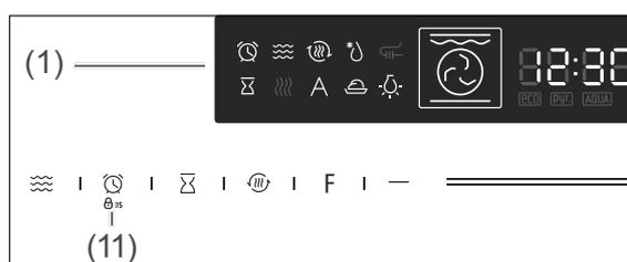
Your oven is equipped with a child lock which protects against the oven being used without permission or unintentionally switched on or off or the settings being changed.
