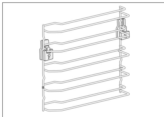
3. Ensure that the baking tray guides are sitting in their brackets on both sides and do not touch the inner cooking compartment wall.
