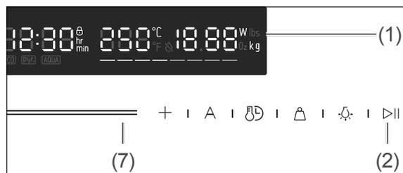
3. To enter a start hour from 0 to 23, use the +/- sensors or the slider (7).
