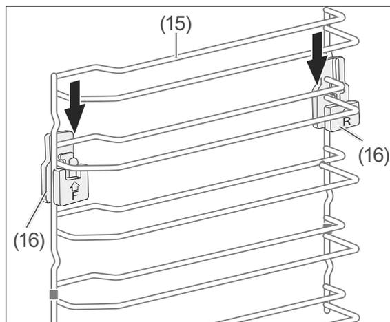
1. Insert the baking tray guides (15) from the side into the brackets (16).
