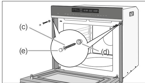
3. If the oven is correctly set up, open the oven door and screw it to the built-in cupboard using the included assembly material. Use the spacers (d), the screws (c) and the blind plugs (e)
