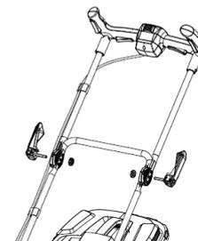
When unfold the mower avoid pinching or trapping any cables!
