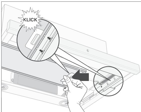
5. Place a grease filter with the pins into the openings on the left side.
