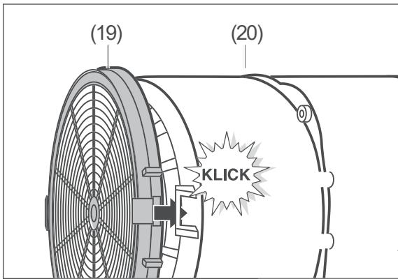
5. Place the new activated charcoal filters on the left and right side of the motor: Put the holding lug into the rectangular opening, place the filter onto the motor, and let the locks click into place.
