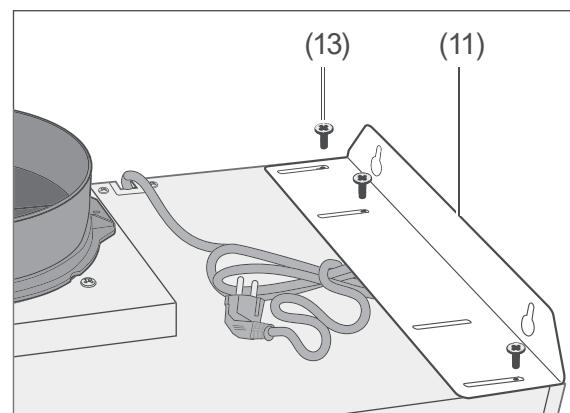
1. Turn the six screws (13) through the retaining plate (11) into the corresponding openings on the exhaust hood.
