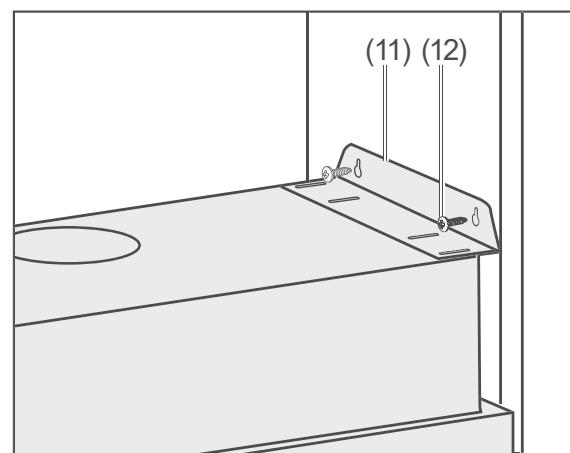
2. Position the exhaust hood in the desired position and screw the two retaining plates (11) tightly into the side walls of the recess using the four screws (12).
