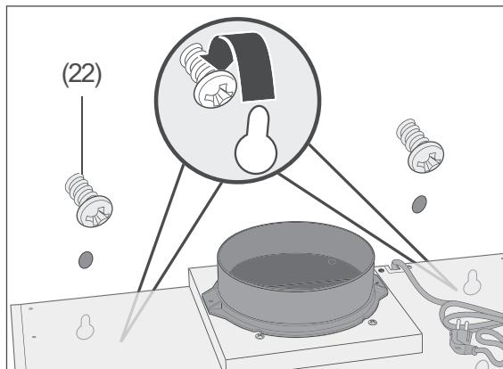
2. Screw the two round-head screws measuring 4.0 × 30.0 mm for the keyhole openings (22) for hanging the Exhaust hood into the wall plugs. There must be enough space between the wall and the heads of the screws so that the Exhaust hood exhaust hood can be hung by the keyhole openings.
