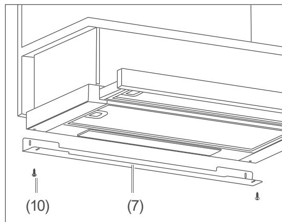
3. To ensure the exhaust hood is firmly anchored, turn the screws (10) through the openings of the holding plate (7) from below.
