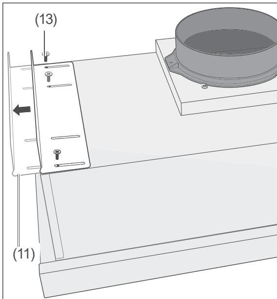
3. Adjust the exhaust hood so that it is centred within the recess and then tighten the six screws (13).
