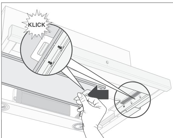
6. Place a grease filter with the pins into the openings on the left side.
