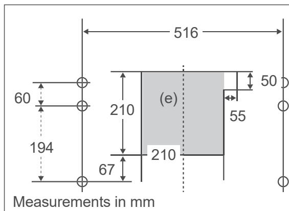
2. Cut a rectangular opening (e) of 210 × 210 mm. Observe the lateral distances shown in the illustration above.
