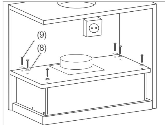
2. Insert the exhaust hood and use the six screws (9) and washers (8) to fix it in place.
