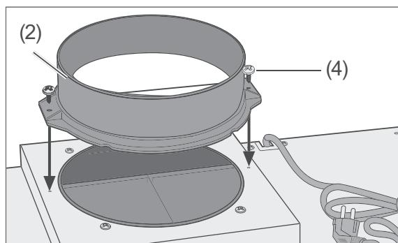
Regardless of whether the exhaust hood is to be mounted on a wall or in a hanging cabinet, the plastic holder and check valve must be mounted.
