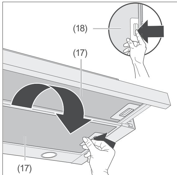
3. Open the lock (18) on the grease filters (17), and carefully pull the grease filters (17) downwards to remove them.
