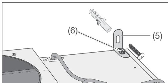
1. Screw the two angle brackets (5) with the screws (6) into the openings on the top of the exhaust hood.
