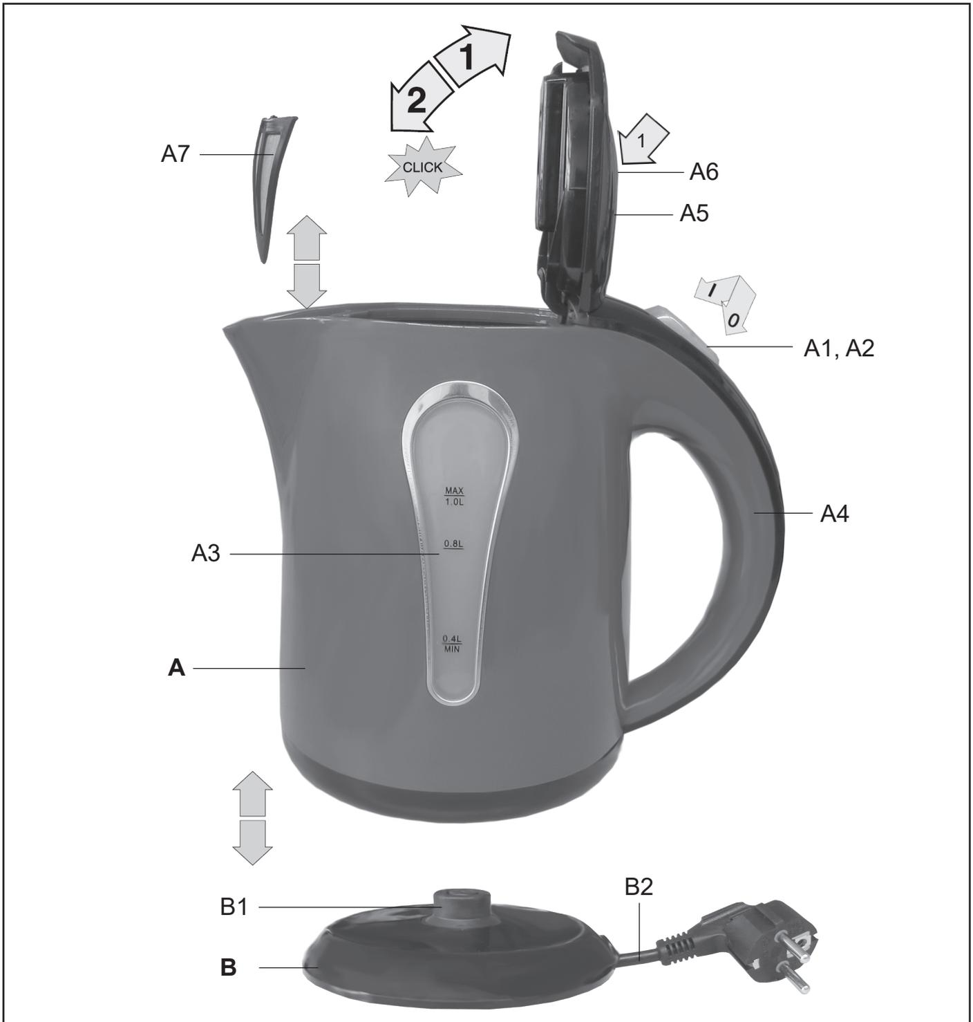
Put the electric kettle on the stand and turn it to the **I** position by the **A1** button. Function of the electric kettle is signaled with the control light **A2**. After boiling the appliance switches off automatically. Before reaching the boiling point, you can switch off the appliance by turning the **A1** button to the **0** position. Always use fresh drinking water for boiling.
