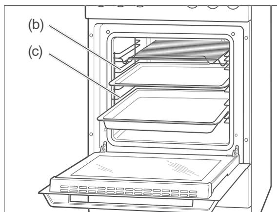
The supplied baking tray (b) and the dripping pan (c) both have an angled edge. Please ensure that this edge is facing forward on being placed in the oven.
