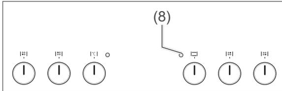
The yellow power indicator light (8) is illuminated as soon as at least one of the solid plates or the oven is switched on. It will switch off again when **all** of the solid plates **and** the oven are switched off.
