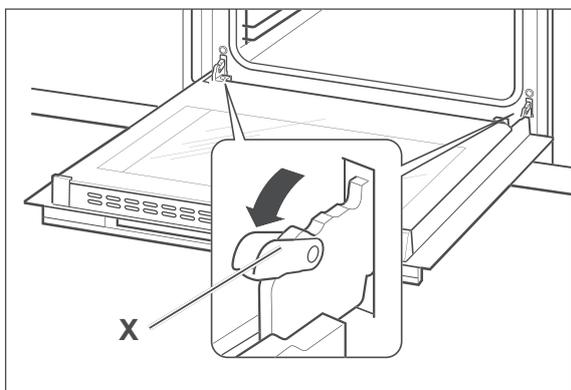
2. Fold the clips **X** on both sides all the way forward. Use a screwdriver if necessary.
