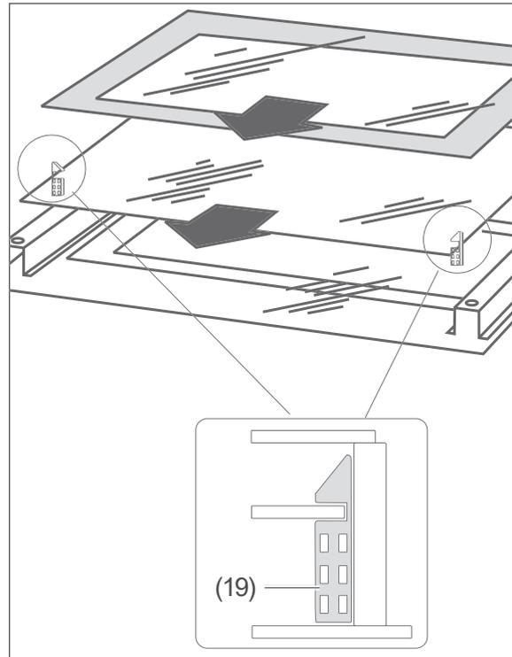
4. Remove the upper pane from the mounts below the hinges and carefully set it down.
