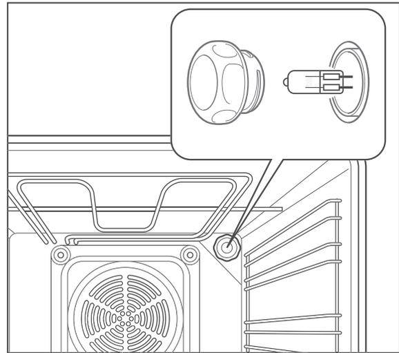
3. Unscrew the glass cover anticlockwise and remove it.
