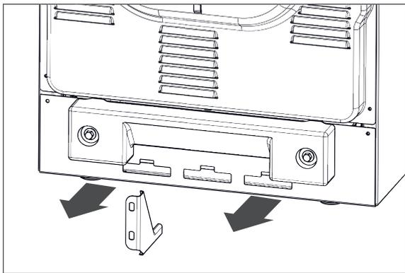
9. Slide the cooker into place and check that the tilt protection prevents the cooker from tipping forward.
