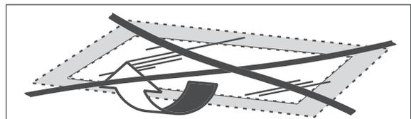
11. Reposition the upper pane in the mounts at the hinges. Make sure that the smooth side is facing outwards.
